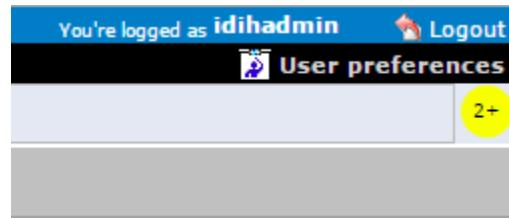
Selecting the alarm status indicator shows a brief description of the open alarms. The system displays the list of open alarms in tabular form, as shown in Figure 3-2. This list can be dismissed by pressing the **Close** on the Open Alarm dialog window.
